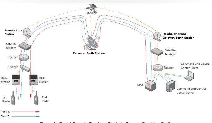
Figure 2: Test 1 Remote Trunking Radio to Remote Trunking Radio
