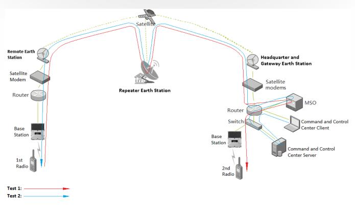
Figure 3: Test 2 Remote Trunking Radio to Local Trunking Radio
