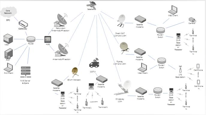
Figure 4: Digital Radio Systems over Satellite Components
