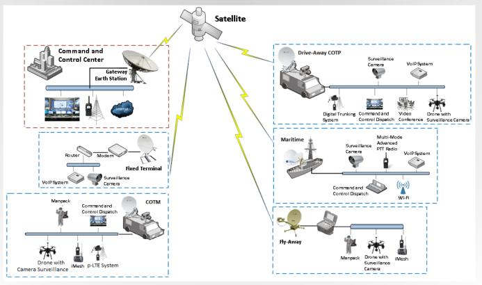
Figure 6: Representative Satcom Solution with Different Types of VSAT
